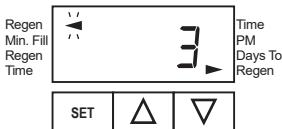
If the system has called for a regeneration that will occur at the preset time of regeneration, the arrow will point to Regen.
