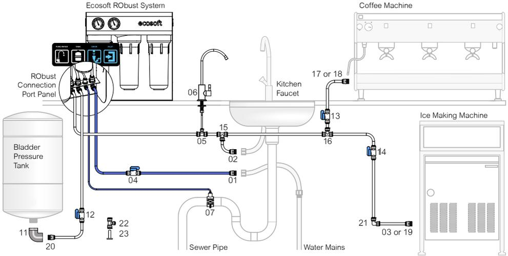
Some of the fittings shown on the diagram come from RObust package. These fittings can be used interchangeably or together with the fittings from RObust connection fitting pack when it's necessary to connect more than one appliance with 3/8" or 1/2" female thread ports or a 3/4" pressure tank. If any of your appliances have different thread sizes, use a suitable adapter for connecting it.
